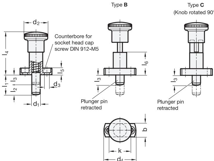
**3 Type****B** without rest position**C** with rest position
