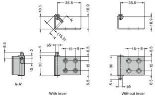
For right-hanging, the hinge with lever is at the upper side, while that without lever at the lower side.
