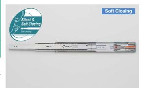
Soft-closes at 20mm distance from closed position (slide length 350mm or below) or 36mm distance from closed position (slide length 400mm or above).
